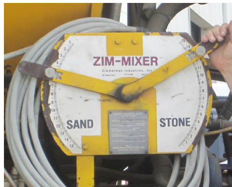
Figure 3. Volumetric batch truck gate setting controls
